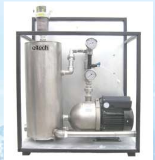
Ozone Injection Skid
